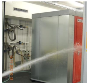
...Water jet test ...
